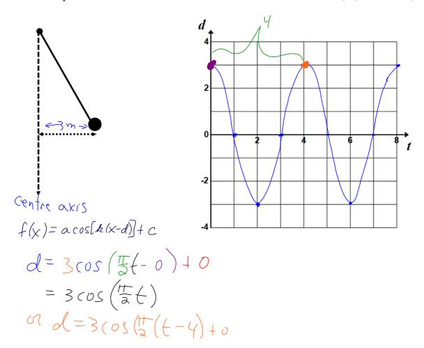
$$|\alpha| = \frac{\text{max-min}}{\text{period}} \quad |\beta| = \frac{\text{orig}}{\text{period}} \quad d = 0 \quad c = \frac{\text{max+min}}{2}$$
