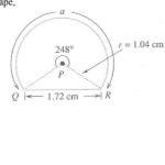
b) If the cam is 0.36 cm thick and is made from an alloy whose density is 3.8g/cm<sup>3</sup>, determine the mass of the cam. (to 3 decimal places)
